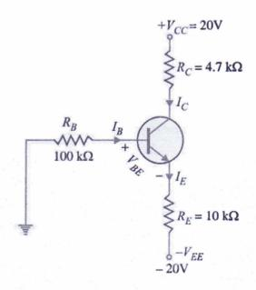
d) Calculate the emitter current in the voltage divider circuit shown below. Also find the value of  $V_{CE}$  and collector potential. (4 Marks)
