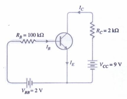
c) For the emitter bias circuit shown below, find  $I_E, I_C, V_C$  and  $V_{CE}$  for  $\beta$  = 85 and  $V_{BE} = 0.7 \, V. \tag{4 Marks}$
