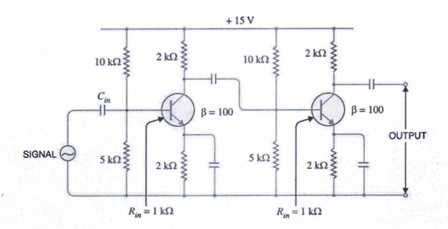
If the input resistance  $R_{in}$  of each stage is 1 k $\Omega$  and  $\beta$  = 100, find:
