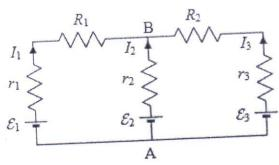
Take  $\mathcal{E}_1 = 6 \text{ V}$ ,  $r_1 = 1\Omega$ ,  $\mathcal{E}_2 = 10 \text{ V}$ ,  $r_2 = 2\Omega$ ,  $\mathcal{E}_3 = 12 \text{ V}$ ,  $r_3 = 3\Omega$  and  $R_1 = R_2 = 20\Omega$ .
