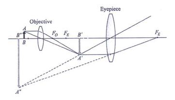
Determine total magnification, if the eye is held close to the eye piece and views virtual image AB at a distance of 25cm. (3 Marks)
